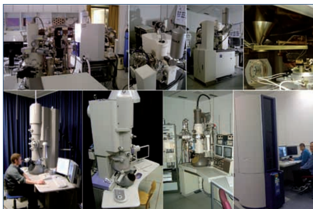
Equipment at EMEZ: upper row FIB/SEM and HRSEM and a view into a cryo-SEM chamber. Lower row cryo and analytical TEM and a dedicated Cs corrected STEM (EMEZ).
